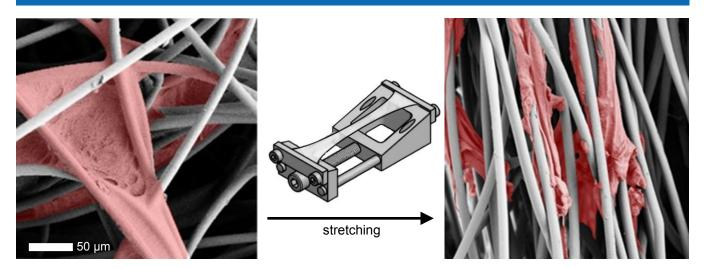
Fig 1. (*left*) False colour electron microscope image of unstretched scaffold visualizing the connection between the PGA and P4HB polymers, (*middle*) stretching the elastic scaffold, (*right*) stretched scaffold with aligned fibres [1]
